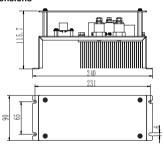
Fig C.2 Switching module installation dimensions (unit: mm)
