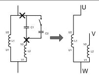
U1 and V1 are the common terminals of the windings. Connect them to the output terminal W of the solar pumping inverter. Connect U2 to the output terminal U of the inverter. Connect V2 to the output terminal V of the inverter. (Note: Use the screws equipped with the inverter.) Connect S4 of the inverter to COM in short circuited manner.
