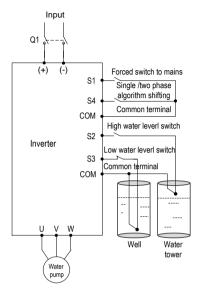
Fig 3.3 Standard wiring diagram
